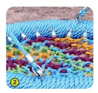
**2- The pod** is made from Usacord Long-Life rope, Ø 16mm. The rope is composed of 4 plaited cords, each made up of six, Ø 2mm, galvanised steel cables.
