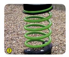
2- The springs are made from Grade 35SCD6 steel, shot blasted, stress relieved, zinc coated and finished with two coats of epoxy polyester powder.
