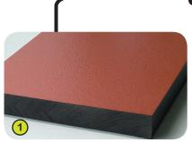
1- The coloured panels are made with a compact material 13mm thick. It is made up of 70% of softwood fibres and 30% of thermosetting resin, and it stands up to weathering very well (sun, rain, damp, etc.). The coloured surfaces are treated with products based on coloured acrylic polyurethane resins; this enables them to stand up well to UV radiation and resist damage.
