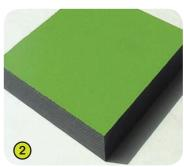
2- The coloured panels are made with a compact material 13mm thick. It is made up of 70% of softwood fibres and 30% of thermosetting resin, and it stands up to weathering very well (sun, rain, damp, etc.). The coloured surfaces are treated with products based on coloured acrylic polyurethane resins; this enables them to stand up well to UV radiation and resist damage.
