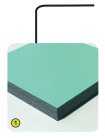
1- The coloured panels are made with a compact material 13mm thick. It is made up of 70% of softwood fibres and 30% of thermosetting resin, and it stands up to weathering very well (sun, rain, damp, etc.). The coloured surfaces are treated with products based on coloured acrylic polyurethane resins; this enables them to stand up well to UV radiation and resist damage.
