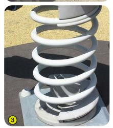
3- The springs are made from Grade 35SCD6 steel, shot blasted, stress relieved, zinc coated and finished with two coats of epoxy polyester powder.
