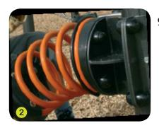
2- The springs are made from Grade 35SCD6 steel, shot blasted, stress relieved, zinc coated and finished with two coats of epoxy polyester powder 100 microns thick. Proludic have patented an exceptionally strong and secure polyamide fixing for the spring ensuring long product life and exceptional levels of safety.
